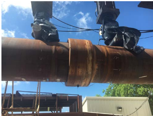
Figure 1: Bend Testing Rig for Monolithic Isolation Joint
