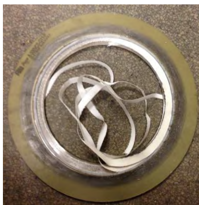
Figure 9: Gasket Exposure to Steam (10)
