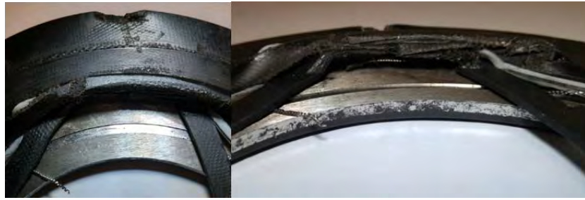
Figure 13: Gasket samples of GRE at High Pressures
