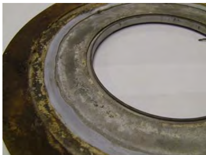
Figure 10: High Temperature exposure of G10 (11)
