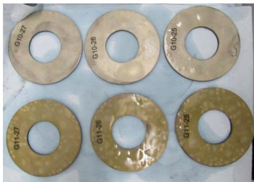
Figure 8: G10/G11 After Sour Gas exposure - 14 days (8)
